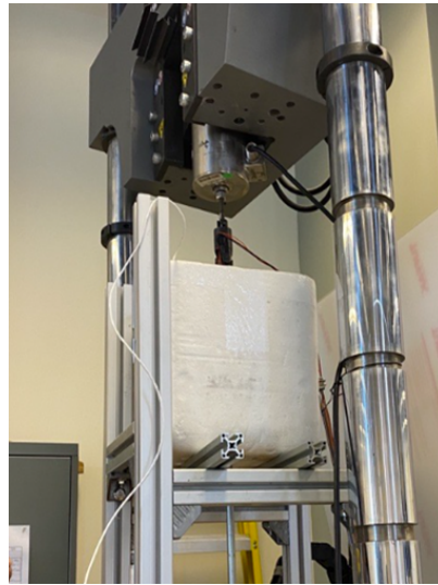
Figure 2: Loaded specimen setup for cryogenic temperature testing, showing the specimen mounted in the grips, instrumented with electrodes, and fully submerged in liquid nitrogen.
